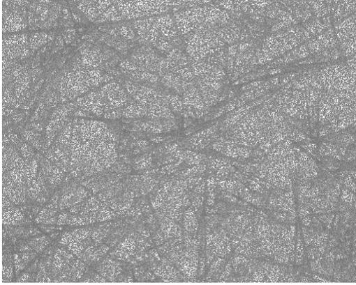
**Figure 5.** Scanning Electron Microscope photo of a grouping of the ACM silicon carbide single crystals.
