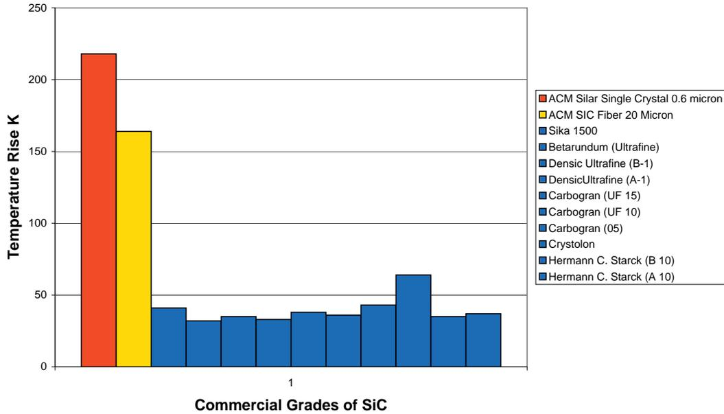
Figure 4. Temperature Change of SiC in Microwave Field.
