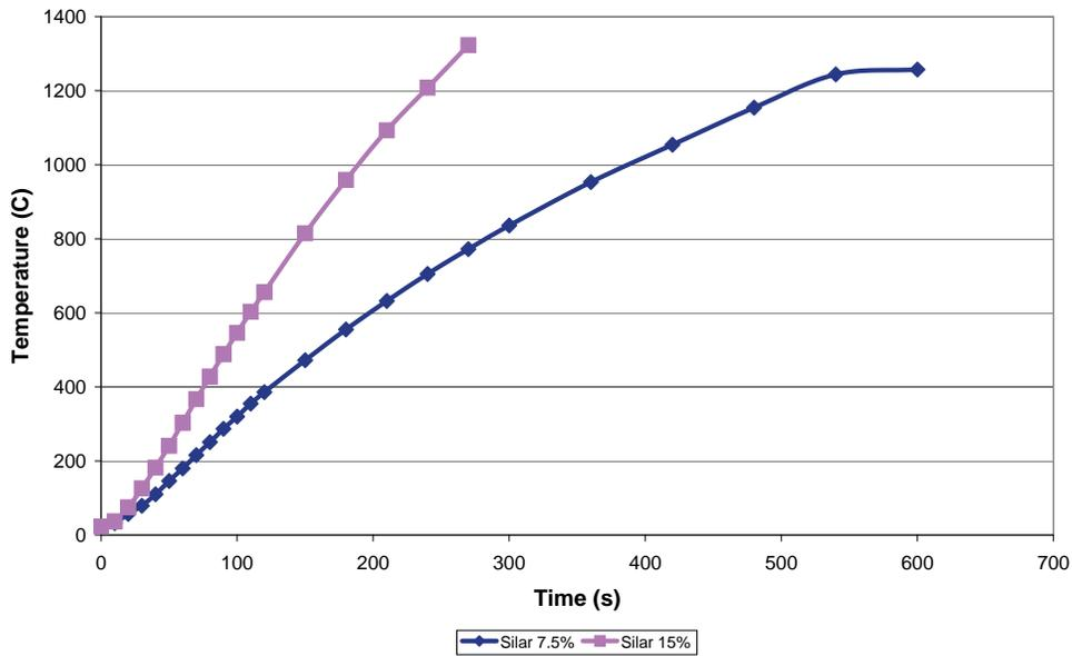
*Figure 2. Heating Rate vs. Silar Loading Level.*
